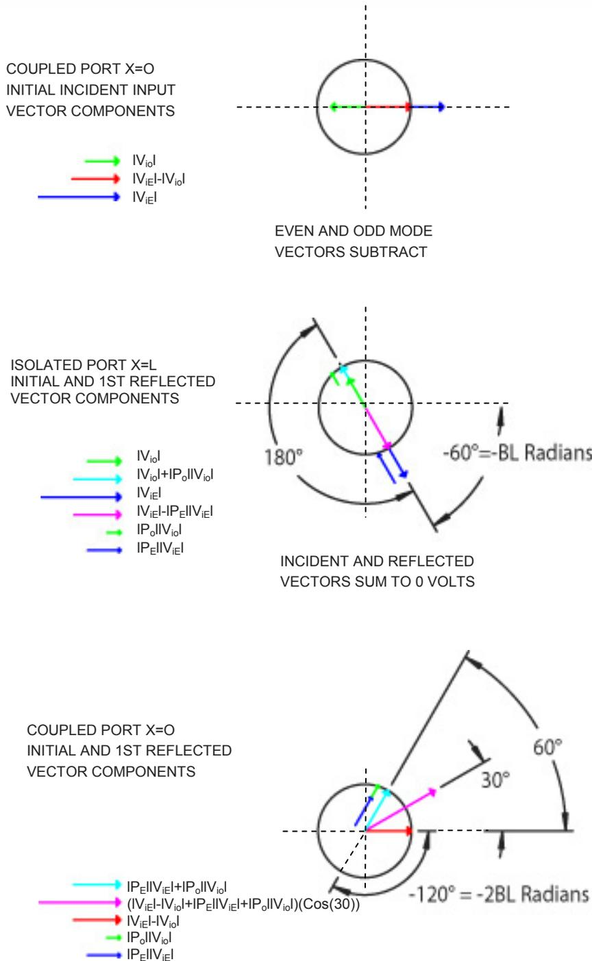
EQUAL INCIDENT AND REFLECTED VECTORS ADD AND THE ANGLE BETWEEN THEM IS DIVIDED BY 2. AS L INCREASES BL RADIAN APPROACHES 90 DEGREES AND THIS ANGLE GOES TO 0 DEGREES RESULTING IN MAXIMUM COUPLED OUTPUT.
