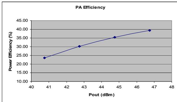
Figure 7: PA drain power efficiency Vs. output power
