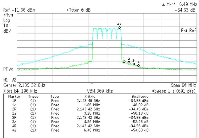
Figure 10-A: TD-SCDMA: Pre (blue) and post (green) DPD spectral plots at 46dBm Pout and 8dB PAR
