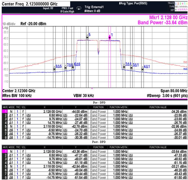
Figure 9-A: WiMax: Pre (red) and post (blue) DPD spectrums at 43.75dBm Pout and 8.5dB PAR
