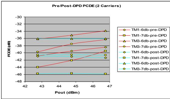
Figure 6-A: PCDE Vs. Pout at different PAR levels and test signals, pre and post DPD
