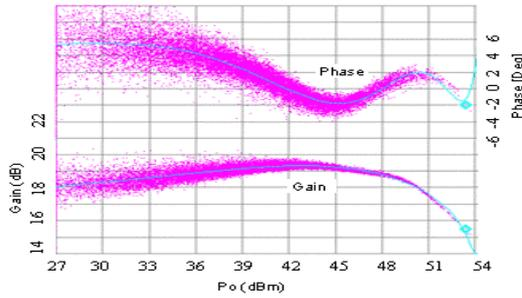
Figure 1: Gain compression and AM-PM characteristics for a typical Doherty PA
