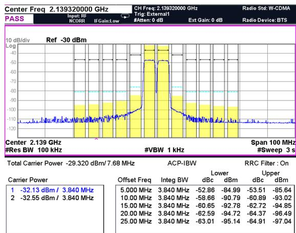
Figure 5-B: Post-DPD spectrum at 46.75dBm Pout and 6dB PAR (TM1-64 data)
