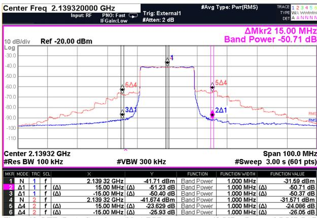
Figure 12: LTE: Pre (red) and post (blue) DPD spectrums at 43.5dBm Pout and 7.5dB PAR
