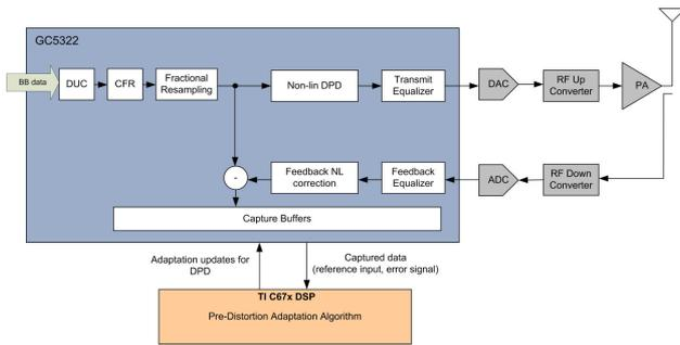
Figure 2: DPD System Diagram
