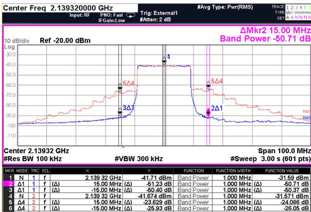
Figure 12: LTE: Pre (red) and post (blue) DPD spectrums at 43.5dBm Pout and 7.5dB PAR
