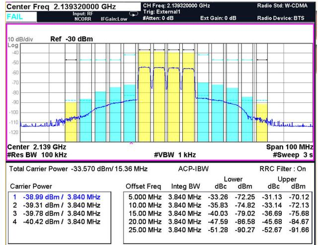
Figure 8-A: WCDMA: Pre-DPD spectrum at 42.75dBm Pout and 6dB PAR (TM1-64 data)
