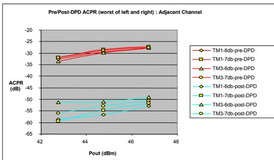
Figure 4-A: Adjacent channel ACLR Vs. Pout at different PAR levels and test signals, pre and post DPD
