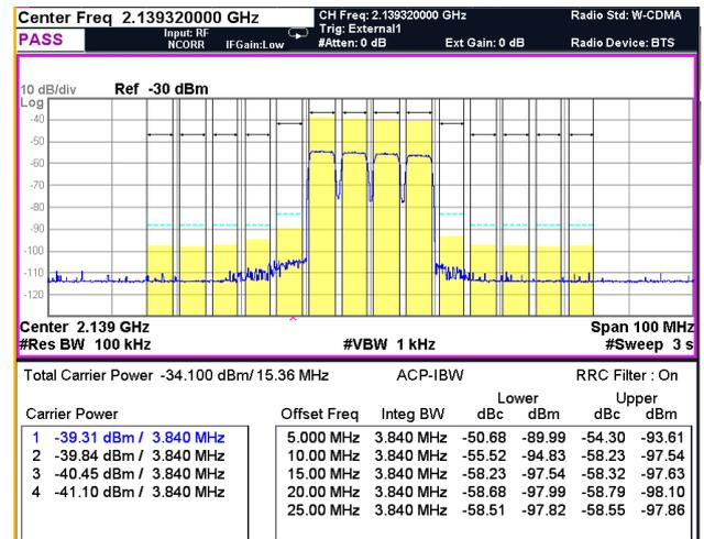
Figure 8-B: WCDMA: Post-DPD spectrum at 42.75dBm Pout and 6dB PAR (TM1-64 data)
