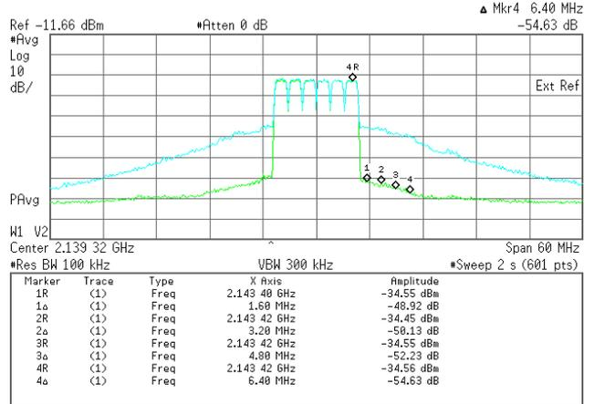
Figure 10-A: TD-SCDMA: Pre (blue) and post (green) DPD spectral plots at 46dBm Pout and 8dB PAR
