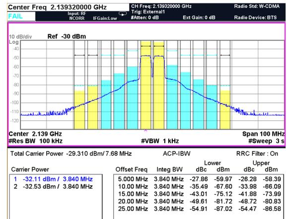
Figure 5-A: Pre-DPD spectrum at 46.75dBm Pout and 6dB PAR (TM1-64 data)
