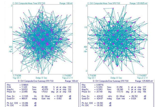
Figure 10-B: TD-SCDMA: Pre-DPD (left) and post-DPD (right) Constellation plots for 46dBm Pout, 8dB PAR
