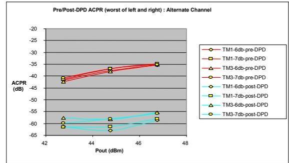
Figure 4-B: Alternate channel ACLR Vs. Pout at different PAR levels and test signals, pre and post DPD
