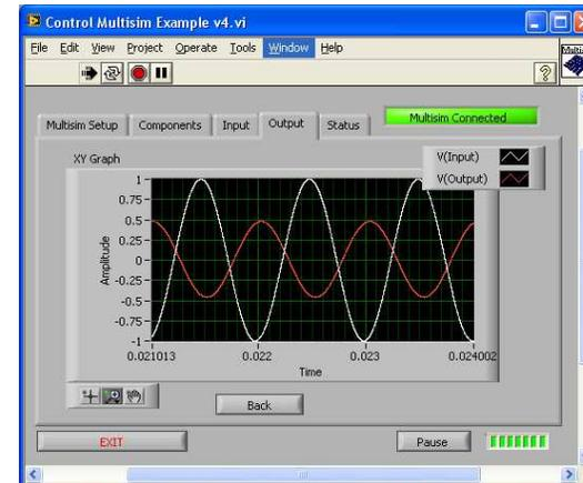
4. Use **LabVIEW VI** to Control Sources and Measure **Test Points** while simulating (similar to DAQ Sampling)
