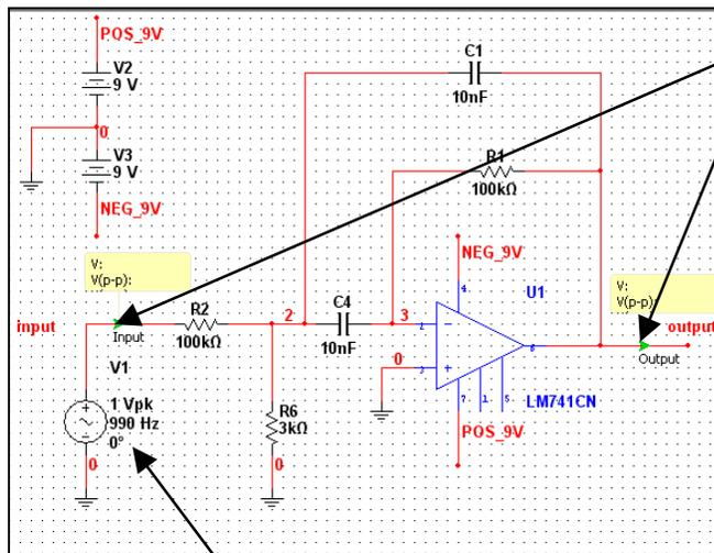
2. Insert appropriate **Test Sources** into Simulation
