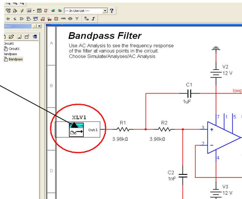
Example showing injection of real hardware test signal into circuit simulation using Virtual Instrument; Exact test pattern can be used on hardware prototype
