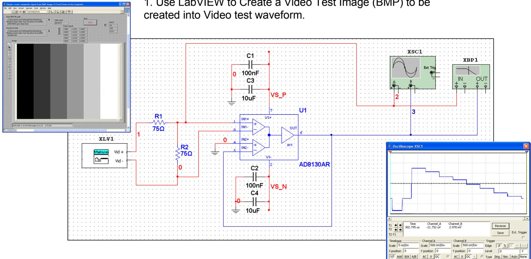
2. Multisim Scope displays video pattern as simulation runs
