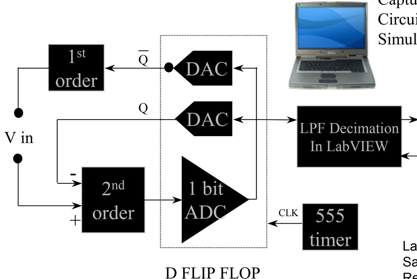
DAQ Card in Laptop Used to Capture Pulse Train from Circuit and Compare Simulation to Measured Data
