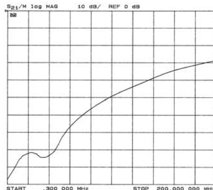
Both ends of shield directly grounded
