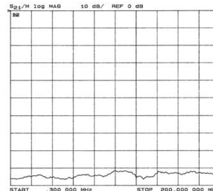
Continuous shield with both ends of grounded directly
