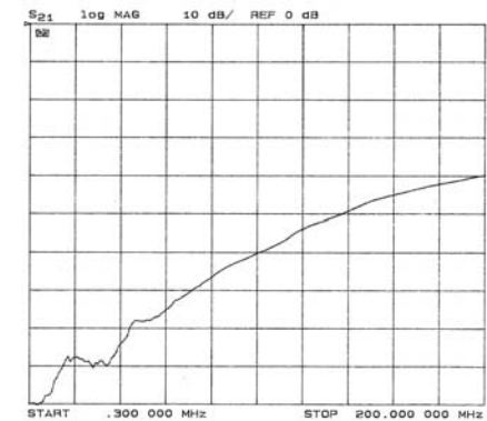
Both shielded ends grounded with 1" loop (19 nH)
