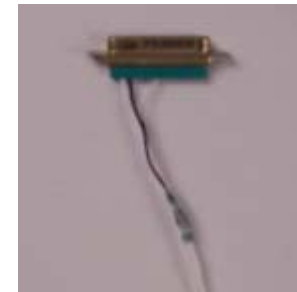
Coax Shield Terminated with Excessive Lead Length
