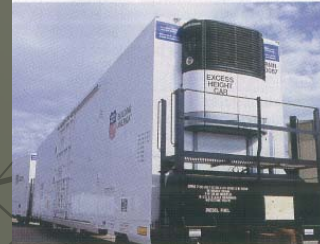
TrinityRail's TRINCool refrigerated car, inside and out. Note the Carrier refrigeration system unit (above). Two photos, TrinityRail
