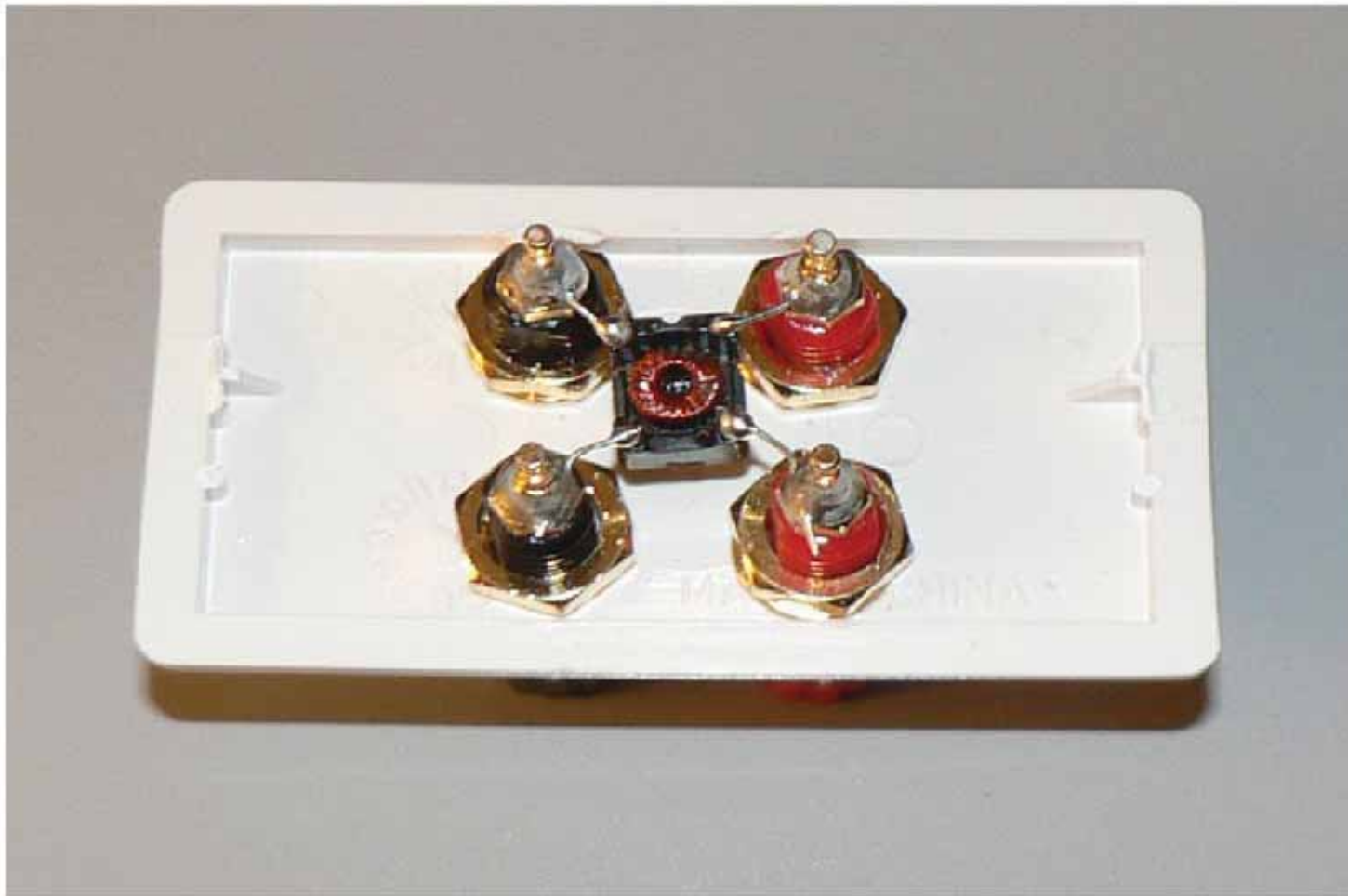
CMC 4.7mH Bifilar Winding
