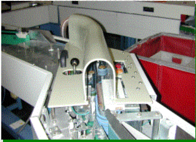
Air Collection System Interfaced To Mail Handling Equipment
