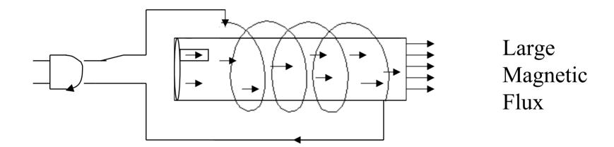
All "small magnets" are aligned in the direction of flux produced by the coil.
