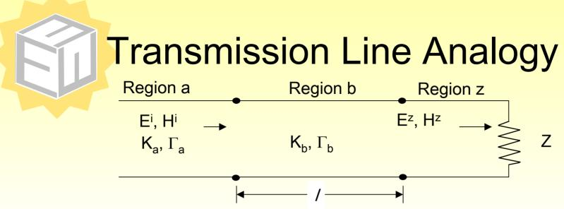
E<sup>i</sup> and H<sup>i</sup> are analogous to voltage and current, respectively, on a transmission line
