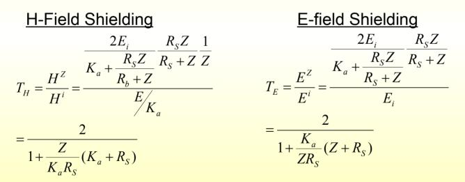
This is an exact model for the low loss case on previous slide
