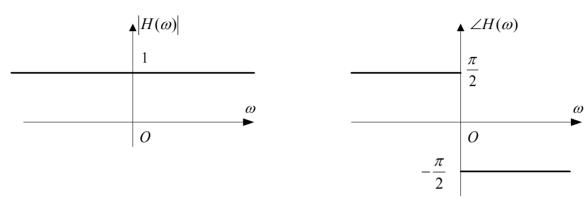
Representation of the transfer function  $H(\omega)$ , an ideal  $\frac{\pi}{2}$  phase-shifter.
