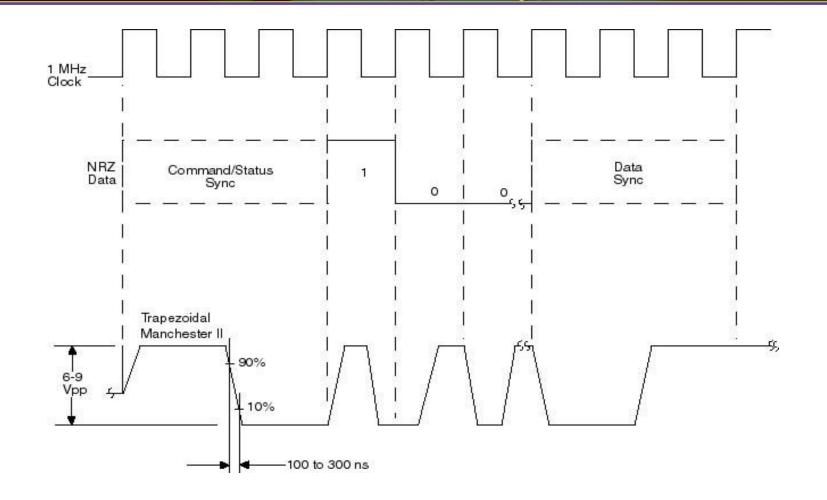
A <u>logic one</u> & <u>logic zero</u> is transmitted as a bipolar coded signal. A transition through zero occurs at the midpoint of each bit time.
