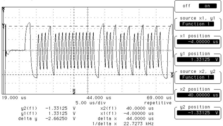
Expanded RT data word. Amplitude of 1.8V at the "Smaller dominant amplitude" (3 boxes).
