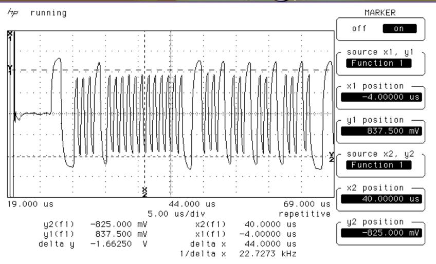
Expanded RT data word with Short Circuit Fault Amplitude of 1.44V at the "Smaller dominant amplitude" (3.6 boxes).
