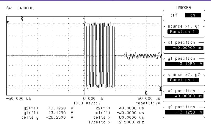
BC Command word amplitude = 26.25V p-p. RT Status word at 400ft. Amplitude = 1.75V p-p. This indicates cable attenuation of almost 3 dB/100 ft (1553 max = 1.5 dB/100 ft).
