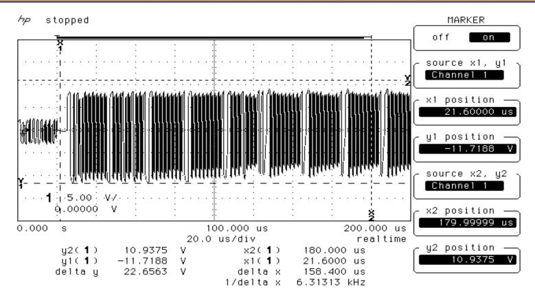
The reason some of our parts seemed OK and some didn't is that the 1553 spec allows rise and fall times of between 100 and 300ns (wide variation). Slow parts passed OK in customers test setup, because of less reflection of harmonics; fast ones don't. But they are all within spec.
