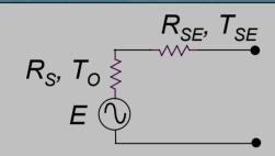
$$F = \frac{N_O}{GkT_OB} = \frac{kT_{SE}B + Gk(T_O - T_{SE})B}{GkT_OB}$$
