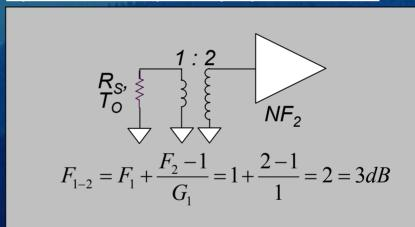
Resistors in input matching networks adversely impact noise figure!
