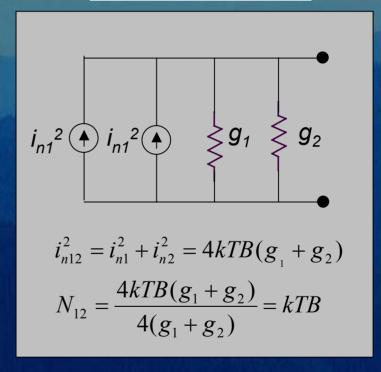
Available noise power from network of resistors at T is still just kTB
