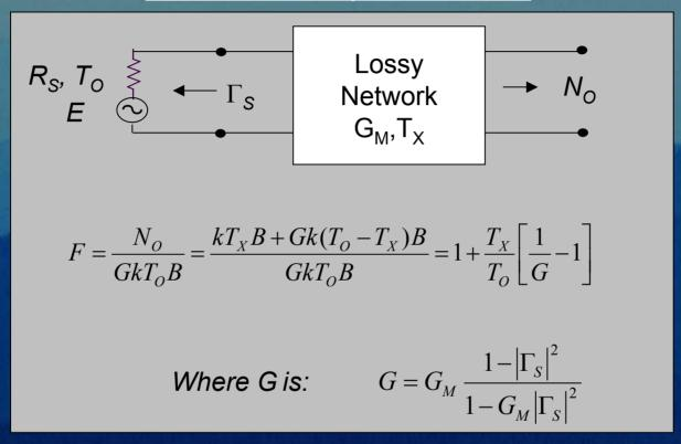
By inspection, F is least when G is greatest ( $R_S$  is matched to the characteristic input impedance of the network  $\Gamma_S$  =0)
