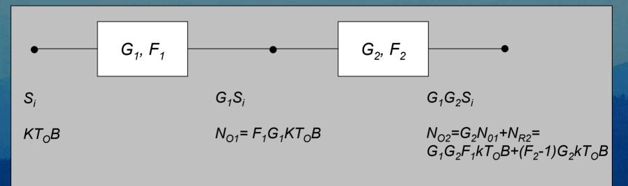
$$F_{12} = \left(\frac{1}{G_1 G_2}\right) \left(\frac{G_1 G_2 F_1 k T_O B + (F_2 - 1) G_2 k T_O B}{k T_O B}\right) = F_1 + \frac{F_2 - 1}{G_1}$$
