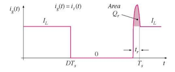
$$\langle i_g \rangle = I_g = (area\ under\ curve)/T_s$$
