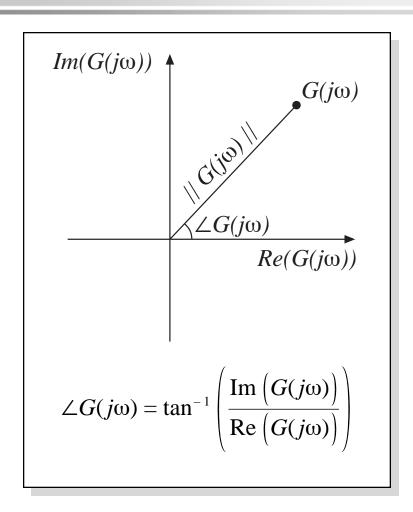
$$G(j\omega) = \frac{1}{\left(1 + j\frac{\omega}{\omega_0}\right)} = \frac{1 - j\frac{\omega}{\omega_0}}{1 + \left(\frac{\omega}{\omega_0}\right)^2}$$
