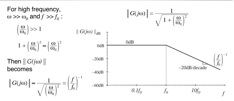
The high-frequency asymptote of  $||G(j\omega)||$  varies as  $f^1$ . Hence, n = -1, and a straight-line asymptote having a slope of -20dB/decade is obtained. The asymptote has a value of 1 at  $f = f_0$ .
