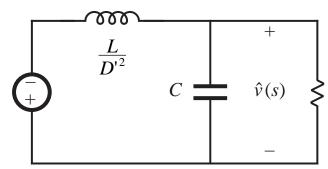
$$\frac{\hat{v}(s)}{\hat{d}(s)} = \left(-\frac{V_g - V}{D'}\right) \frac{\left(R \parallel \frac{1}{sC}\right)}{\frac{sL}{D'^2} + \left(R \parallel \frac{1}{sC}\right)}$$
