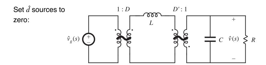
Push elements through transformers to output side:
