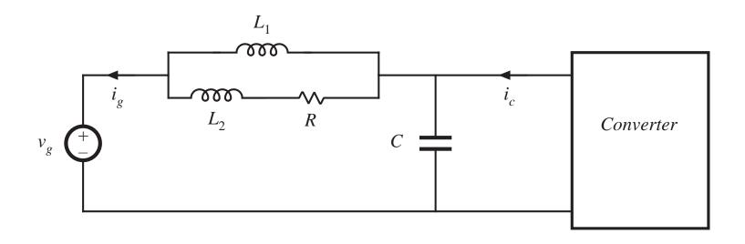
$$G(s) = \frac{i_g(s)}{i_c(s)} = \frac{1 + s\frac{L_1 + L_2}{R}}{1 + s\frac{L_1 + L_2}{R} + s^2L_1C + s^3\frac{L_1L_2C}{R}}$$
