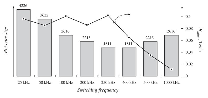
As switching frequency is increased from 25 kHz to 250 kHz, core size is dramatically reduced  As switching frequency is increased from 400 kHz to 1 MHz, core size increases
