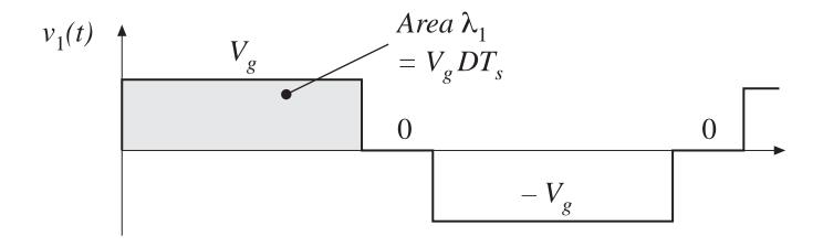
$$\lambda_1 = DT_s V_g = (0.75) (6.67 \,\mu\text{sec}) (160 \,\text{V}) = 800 \,\text{V} - \mu\text{sec}$$
