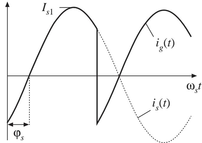
$$\begin{aligned} \langle i_g(t) \rangle_{T_s} &= \frac{2}{T_s} \int_0^{T_s/2} i_g(\tau) d\tau \\ &\approx \frac{2}{T_s} \int_0^{T_s/2} I_{s1} \sin(\omega_s \tau - \varphi_s) d\tau \\ &= \frac{2}{\pi} I_{s1} \cos(\varphi_s) \end{aligned}$$
