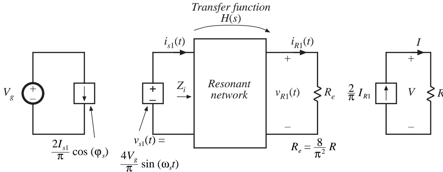
$$M = \frac{V}{V_g} = \underbrace{\left( R \right)}_{\left( \frac{V}{I} \right)} \underbrace{\left( \frac{2}{\pi} \right)}_{\left( \frac{I}{I_{R1}} \right)} \underbrace{\left( \frac{1}{R_e} \right)}_{\left( \frac{I_{R1}}{V_{R1}} \right)} \underbrace{\left( \| H(s) \|_{s=j\omega_s} \right)}_{\left( \frac{V_{R1}}{V_{s1}} \right)} \underbrace{\left( \frac{4}{\pi} \right)}_{\left( \frac{V_{s1}}{V_g} \right)}$$
