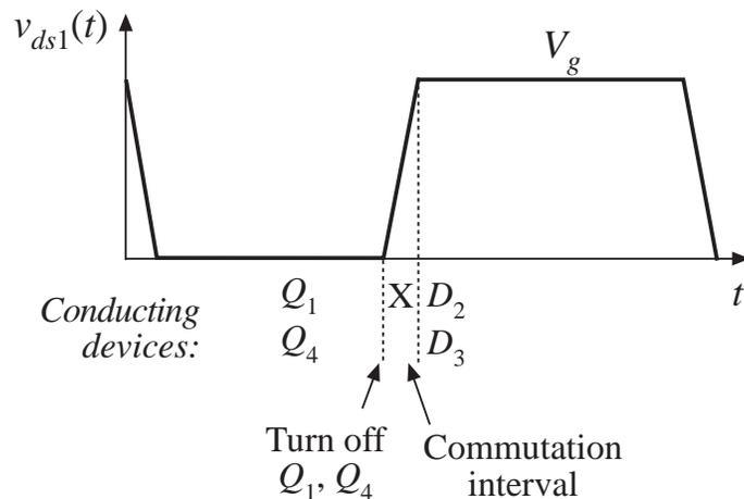
Tank current  $i_s(t)$  charges and discharges  $C_{leg}$ . Turn-off transition becomes lossless. During commutation interval, no devices conduct.
