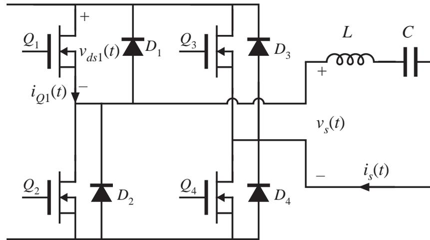
When  $Q_1$  turns off,  $D_2$  must begin conducting. Voltage across  $Q_1$  must increase to  $V_g$ . Transistor turn-off transition is identical to hard-switched PWM. Switching loss may occur (but see next slide).
