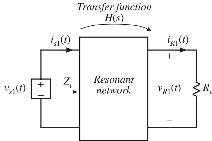
Model of ac waveforms is now reduced to a linear circuit. Tank network is excited by effective sinusoidal voltage (switch network output port), and is load by effective resistive load (rectifier input port).
