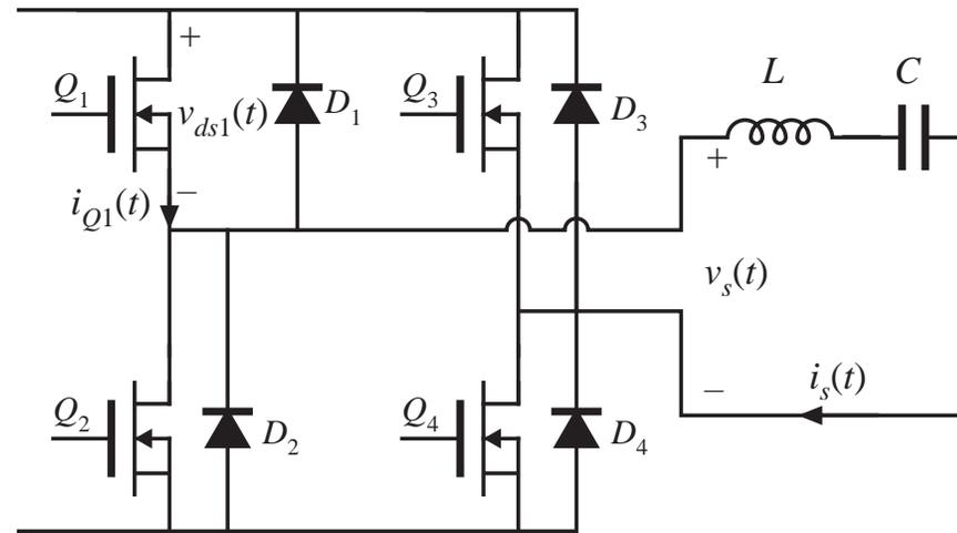
$Q_1$  turns on while  $D_2$  is conducting. Stored charge of  $D_2$  and of semiconductor output capacitances must be removed. Transistor turn-on transition is identical to hard-switched PWM, and switching loss occurs.
