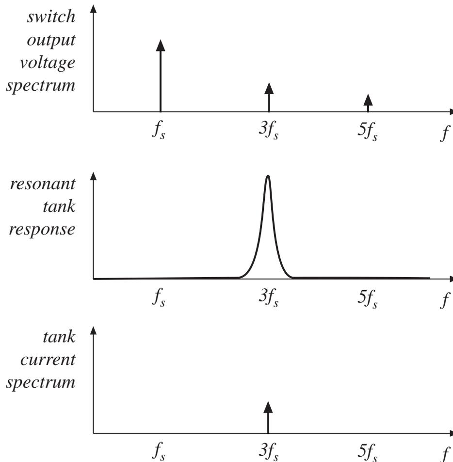
*Example:* excitation of tank by third harmonic of switching frequency
