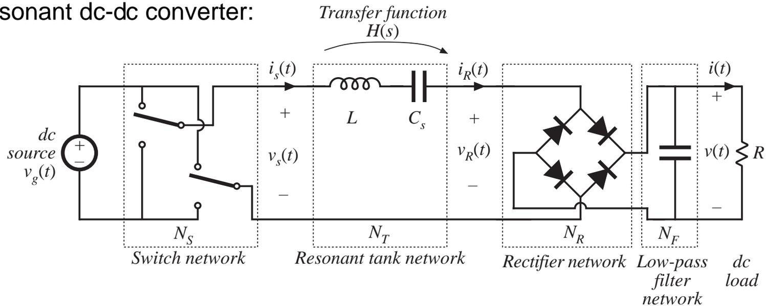
If tank responds primarily to fundamental component of switch network output voltage waveform, then harmonics can be neglected.
