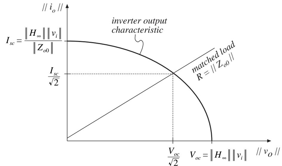
This result is valid provided that (i) the resonant network is purely reactive, and (ii) the load is purely resistive.
