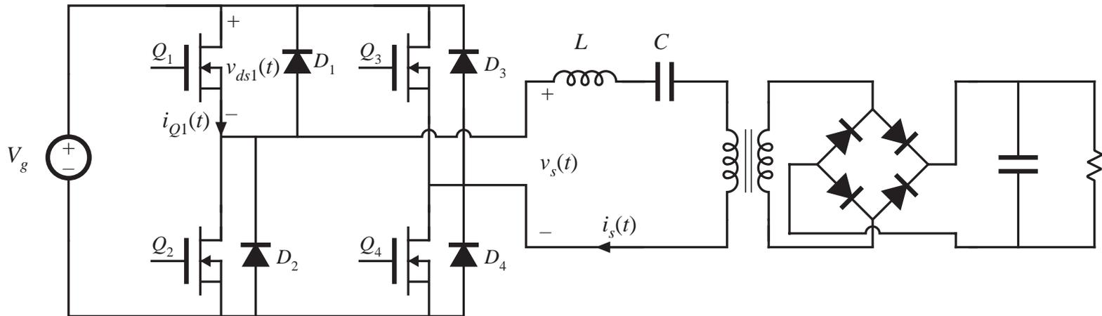
Operation above resonance: input tank current lags voltage
