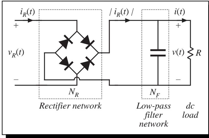
Output capacitor charge balance: dc load current is equal to average rectified tank output current
