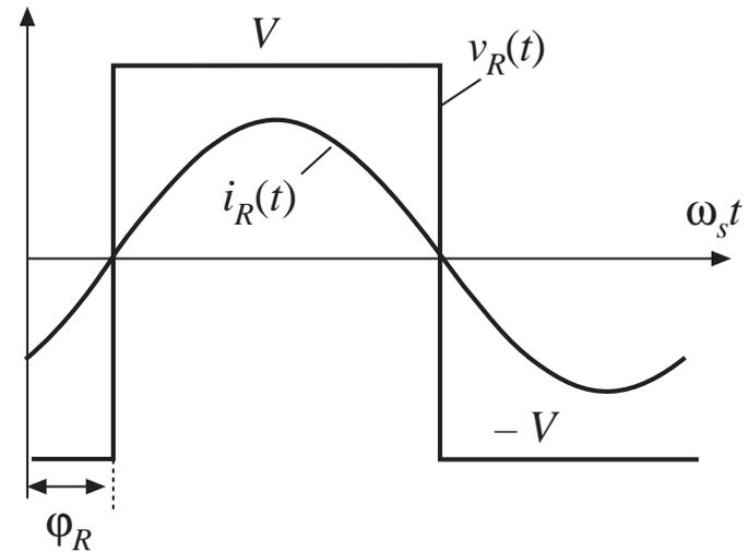
Assume large output filter capacitor, having small ripple.
