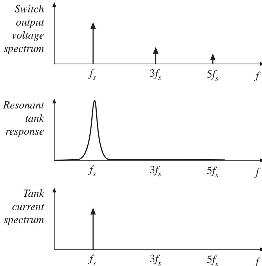
Tank current and output voltage are essentially sinusoids at the switching frequency  $f_s$ .
