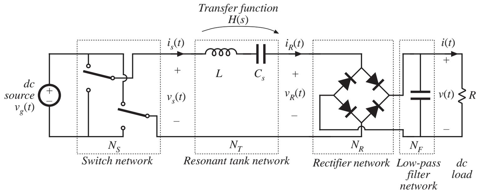
The series resonant dc-dc converter
