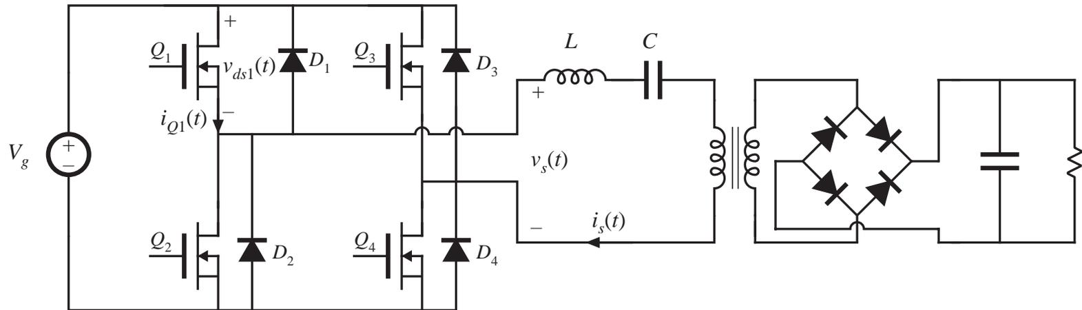
Operation below resonance: input tank current leads voltage
