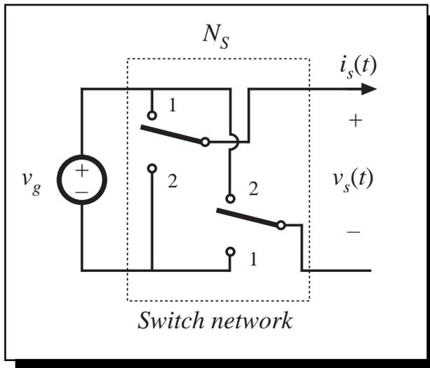
If the switch network produces a square wave, then its output voltage has the following Fourier series:
