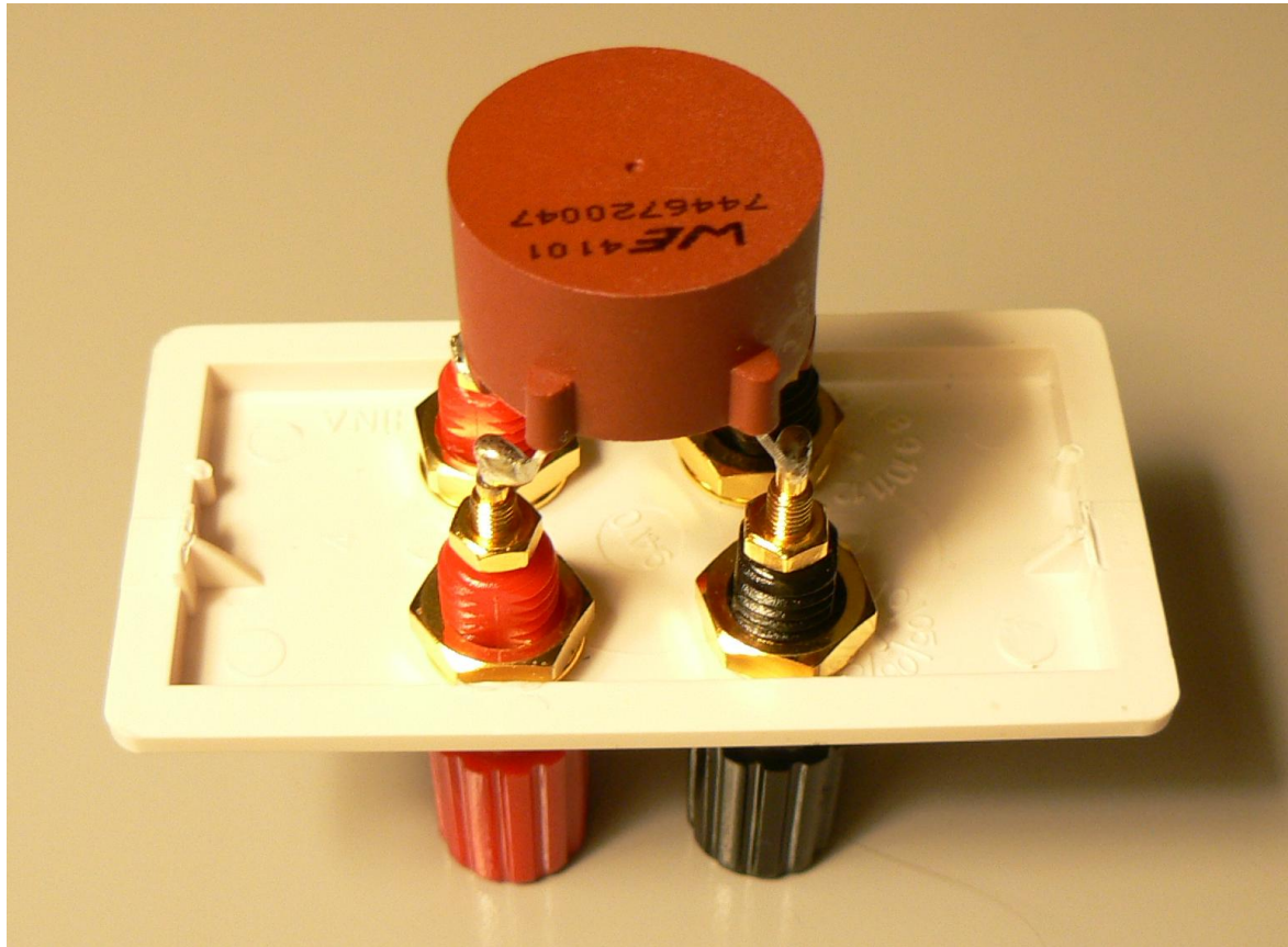
Sectional common mode choke 47mH
