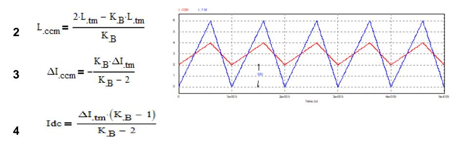
These formulas are used to calculate the inductor parameters as a function of  $K_{\rm B}$  when converting a TM design to CCM
