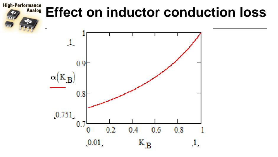
• As expected, lower  $K_B$  (more flux derating) yields lower conduction loss
