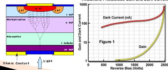
Avalanche Photodiode Gain and Dark Current
