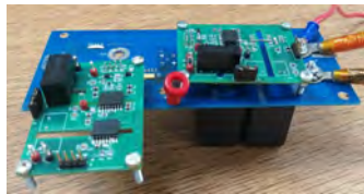
Cryogenic High Density Motor Drive (GaN)
