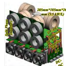
Modular Grid-tied Converter for Grid Control (SiC)
