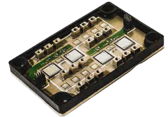
1200V / 350 A HyS TPG Enhanced Thermal Management
