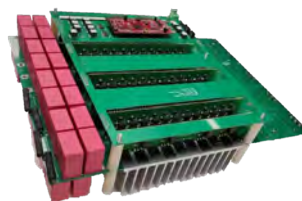
High Density Grid Tied Solar Converter (SiC)
