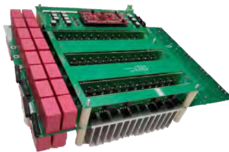
High Density Grid Tied Solar Converter (SiC)
