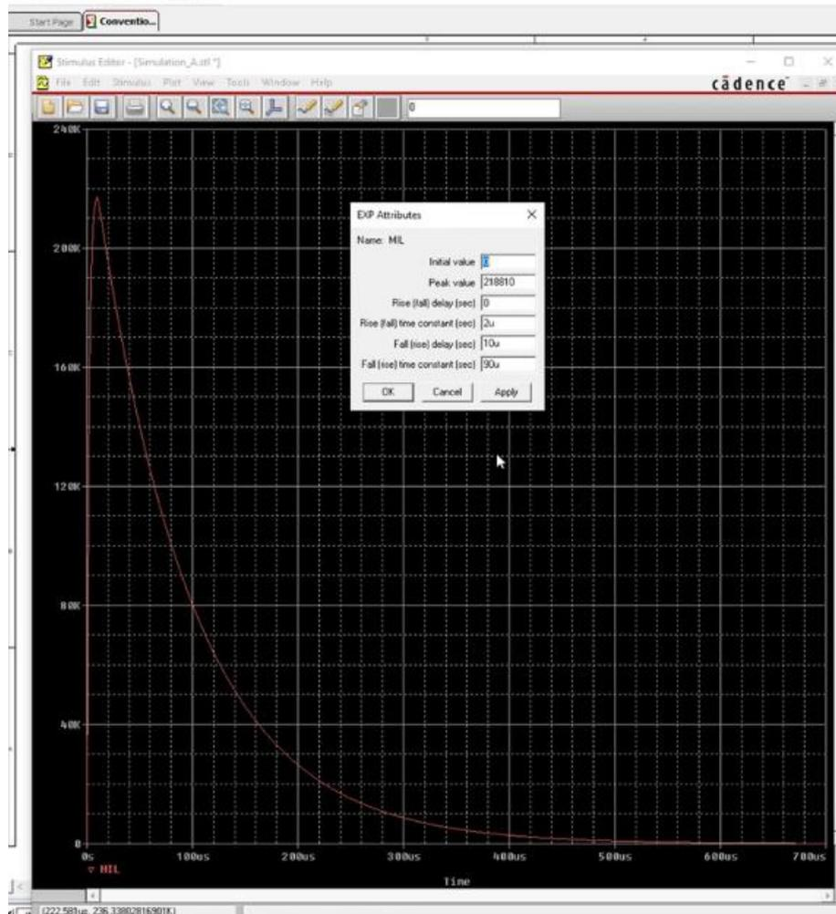
Figure 8 MIL STD component A waveform Pspice Stimulus
