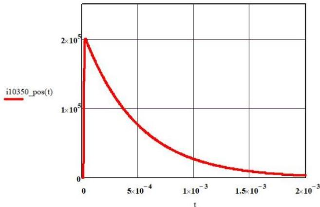
$$Q_{10350\_pos} := \int_{t_{min\_pos}}^{t_{max\_pos}} i_{10350\_pos}(t) dt = 98.543$$
