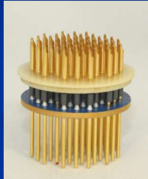
L-FILTER WITHOUT GROUND SPRING
