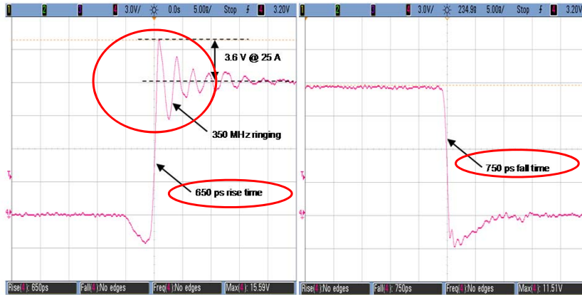
EPC2100 driven by an LM5113 driver IC from Texas Instruments
