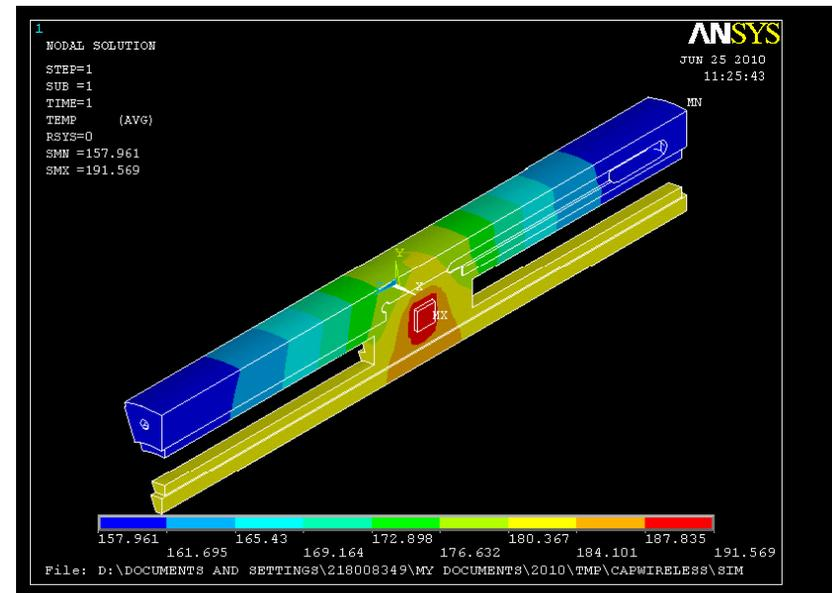
$T_{max} = 192\text{ C}$  (underneath chip)
