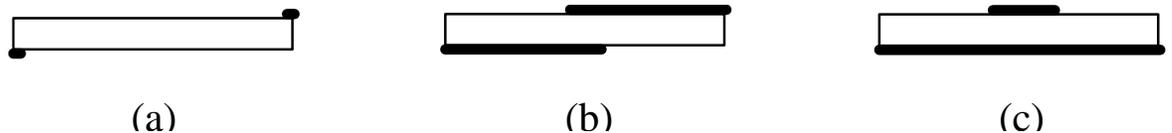
Transforms from 480 Ohms Radiation Element to 50 Ohm microstripline
