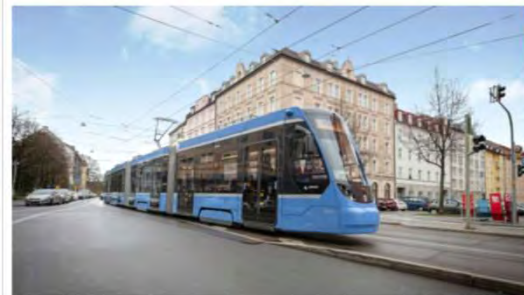
Siemens Mobility and Munich City Authority (SWM) completed a one-year trial in August 2021 using semiconductor technology based on SiC devices fitted to a three-section Avenio LRV
