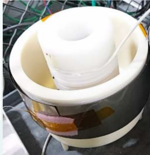
Fig. 2. Two inductively-coupled loops. C2 is parasitic capacitance of transformer/load.
