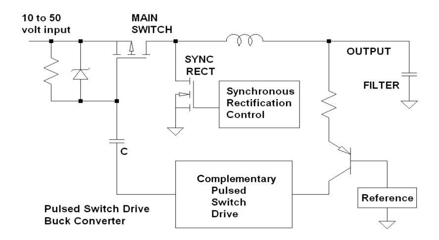
Main switch On time can be constant, or modulated
