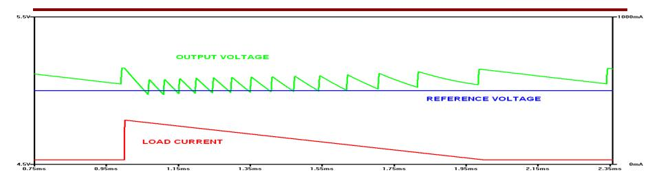
A simple 2-transistor error amplifier running on nextto-no power supply current produces good results
