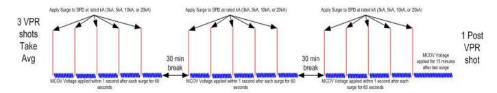
The average of the 3 VPR shots and the Post VPR shot can not vary by more than +/- 10% for the unit under test to pass this test.
