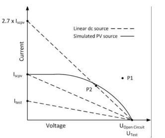
Figure 1. Characteristic Power Source Representations
