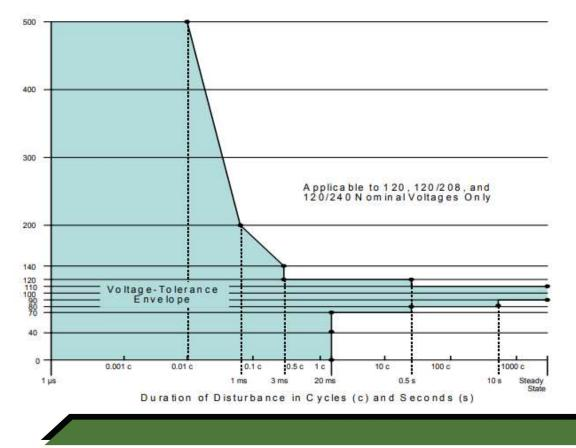
The CBEMA and ITIC curves are both used to visibly represent voltage events. ... It defines various regions based on input voltage where computer equipment may encounter operational issues. The ITIC (Information Technology Industry Council) curve is a modified version of the CBEMA curve created in the 1990's.
