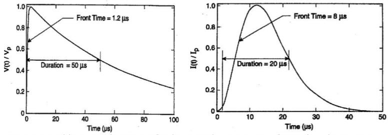
Represented by a combination of voltage and current waveforms (combination wave)
