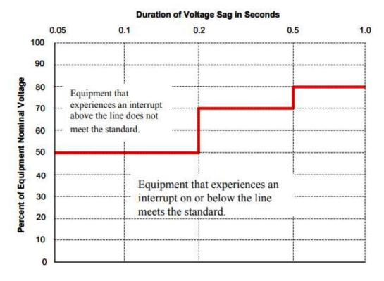
SEMI F47 sets out the required voltage sag tolerance for semiconductor fab equipment; IEC 61000-4-34 is used as the test standard
