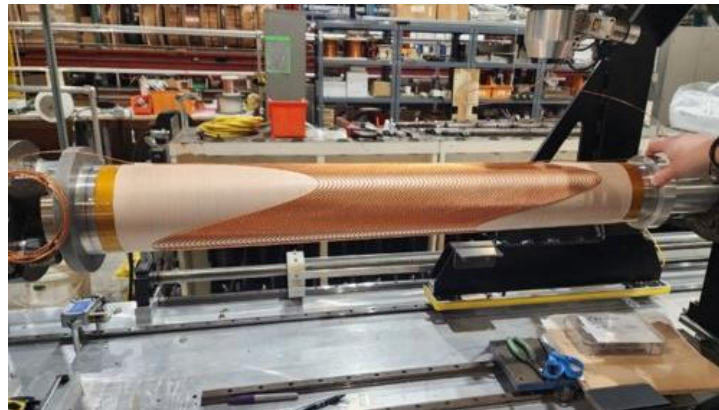
Double Helical Direct Wind Magnet
