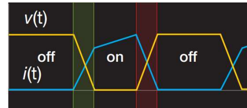
Switch Voltage and Current
