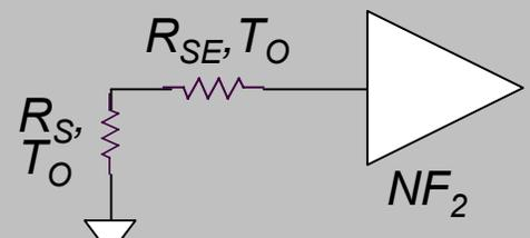
The diagram shows a source with impedance  $R_S$  and noise temperature  $T_O$  connected to a series resistor  $R_{SE}$  and noise temperature  $T_O$ . This combination is connected to an amplifier with noise figure  $NF_2$ .
