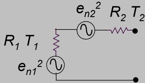
$$e_{n1-2}^2 = e_{n1}^2 + e_{n2}^2 = 4kB(R_1T_1 + R_2T_2) = 4kB[(R_1 + R_2)T_2 + R_1(T_1 - T_2)]$$
