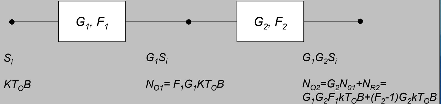
$$F_{12} = \left( \frac{1}{G_1 G_2} \right) \left( \frac{G_1 G_2 F_1 k T_0 B + (F_2 - 1) G_2 k T_0 B}{k T_0 B} \right) = F_1 + \frac{F_2 - 1}{G_1}$$
