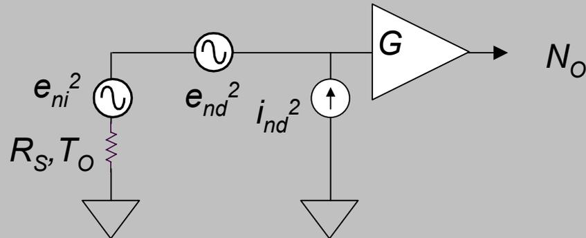
*Output noise power,  $N_{O_i}$ , referenced to input is:*
