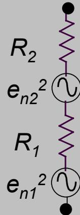
$$e_{n12}^2 = e_{n1}^2 + e_{n2}^2 = 4kTB(R_1 + R_2)$$
