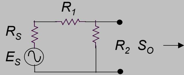
$$G_L = \frac{S_o}{S_i} = \frac{R_s R_2}{(R_1 + R_s)(R_1 + R_2 + R_s)} = \left( \frac{R_s}{R_1 + R_s} \right) \left( \frac{R_2}{R_1 + R_2 + R_s} \right) = G_{SE} G_{SH}$$
