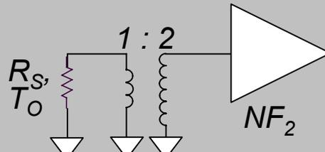
The diagram shows a source with impedance  $R_S$  and noise temperature  $T_O$  connected to a 1:2 step-up transformer. The secondary of the transformer is connected to an amplifier with noise figure  $NF_2$ .
